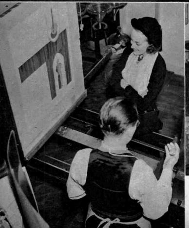
5 These working drawings are placed before a large camera, photographed by Frank Gera (left). He makes a plate for each of the four basic colors in the drawing, develops them himself (above)
