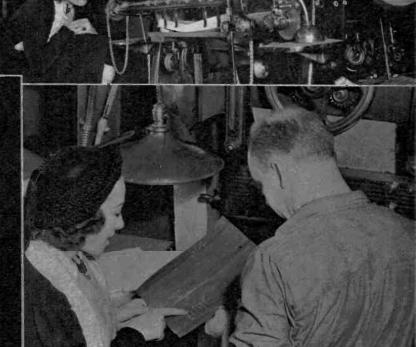
The message for the inside of the card is engraved on a brass block, which is used in the engraving machine operated by George Young, Jr. (above). This machine exerts from 4 to 5 tons pressure on the paper!
