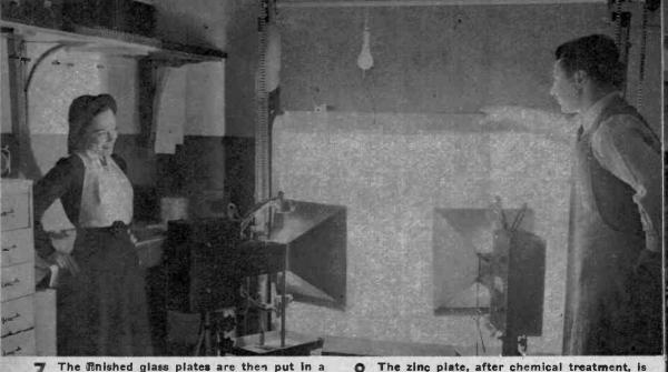
The Mished glass plates are then put in a rack, placed on a sheet of chemically treated zinc. Streng are lights (operated by Hal Aaron, 200ve) burn the image deep into the zinc plate
